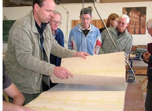
**Applying glue to the edges of the veneer**
